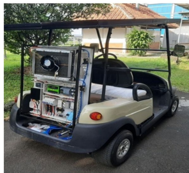
HYBRID CAR BATTERY-PV-FC Use 2.5 kW of PEMFC, 48VDC/3,7kW Motor, PV 200Wp, Lithium Battery 48V/80Ah
