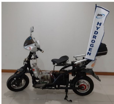
HYDROGEN MOTORCYCLE Use 500 W of PEMFC, NiMH tank 740 L at 150 psi, 48 VDC to 12 VDC controller
