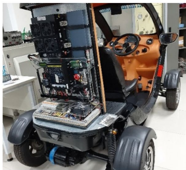
FUEL CELL VEHICLE Use 1 kW of PEMFC, 30V-33.5A, 36VDC/1kW motor, H2-tank 295L/150 bar Compress Cylinder
